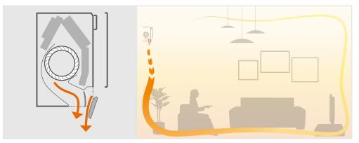
The Coanda effect creates two different airflow patterns depending on whether Stylish is in cooling or heating mode. On the top is the Coanda effect in cooling mode (ceiling airflow), while the bottom images demonstrate the Coanda effect in heating mode (vertical airflow).
